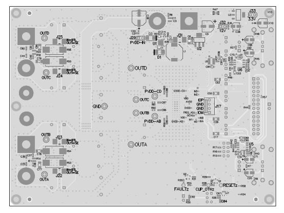
Figure 7. TPA3244EVM Bottom Composite Assembly
