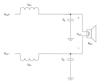
Figure 2. Type-2 Filter for BD or AD Modulation
