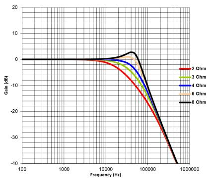
Figure 3. TPA3244EVM LC Filter Cutoff Frequency
