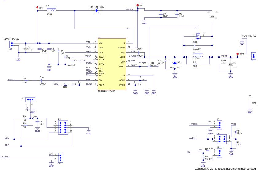
Figure 1. TPS65235-1 EVM Schematic for DiSEqC 2.x Application
