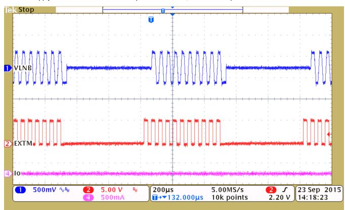
Figure 10. EXTM Has 22-kHz External Tone Input
