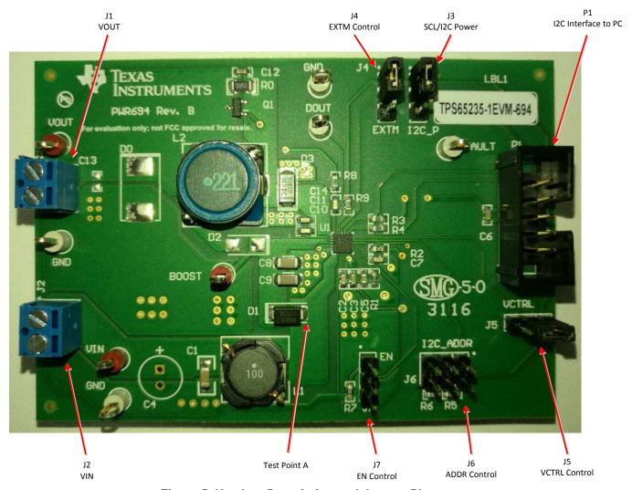
Figure 5. Headers Description and Jumper Placement
