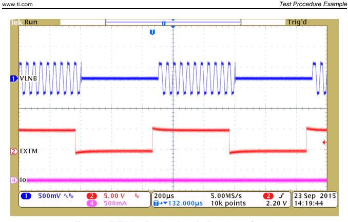
Figure 11. EXTM Has Envelope Input for Tone Output Control
