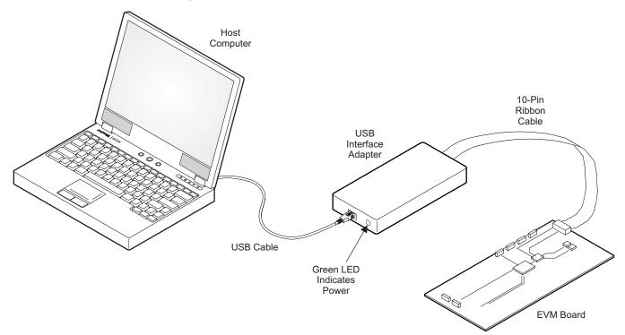
Figure 6. USB Interface Adapter Quick Connection Diagram
