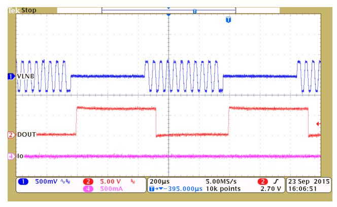
Figure 12. DOUT Output When Tone Received
