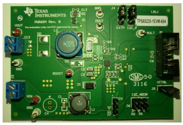
Figure 2. Component Placement (Top Layer)
