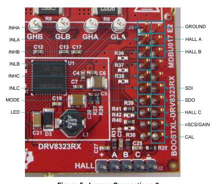
Figure 5. Jumper Connections 2
