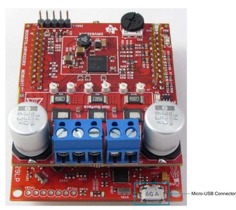
Figure 6. Micro-USB Connection
