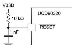
**Figure 1. RESET With R-C Network**
