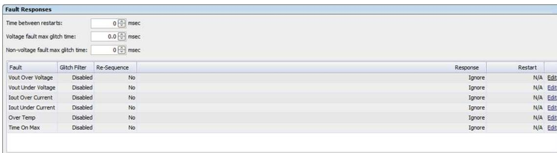
Figure 4-33. Fault Responses Setting For Rest UCD90xxx
