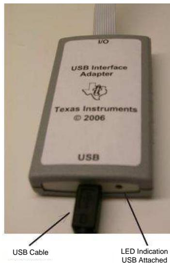
**Figure 2-3. USB-to-GPIO Adapter**
