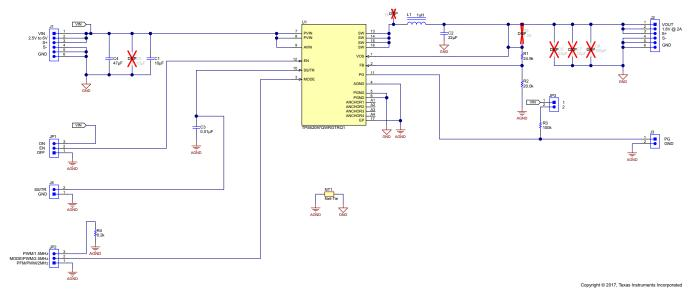
Figure 10. TPS62097QEVM-891 Schematic
