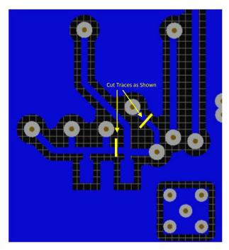
Figure 1. Loop Response Measurement Modification
