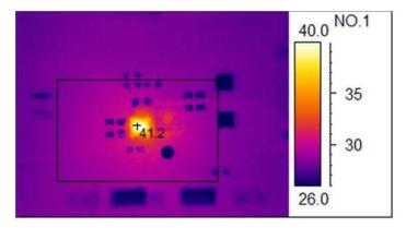
Figure 2. Thermal Performance ( $V_{IN} = 5 \text{ V}$ ,  $I_{OUT} = 2000 \text{ mA}$ , Mode = PFM/PWM)
