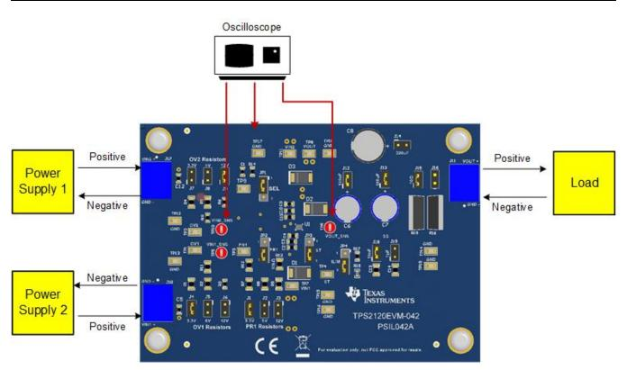
Figure 2. TPS2120 Setup With Test Equipment
