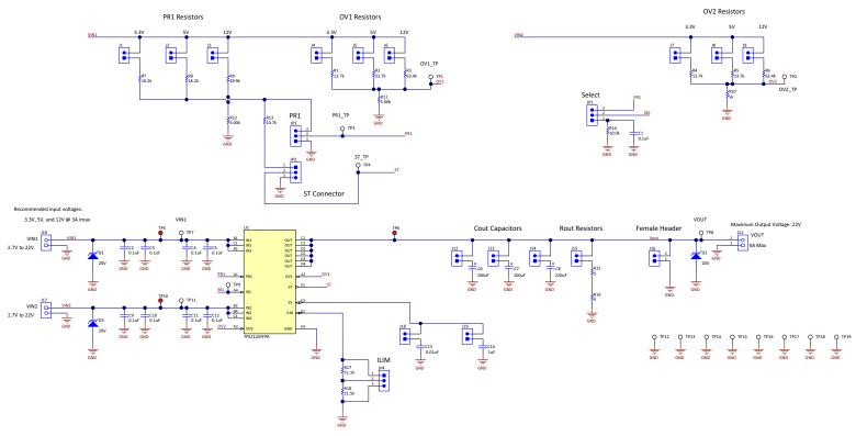
Figure 4. TPS2120 Schematic
