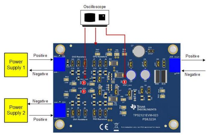
Figure 1. TPS2121 Setup With Test Equipment
