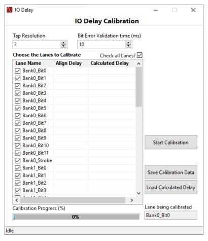
Figure 3-6. IO Delay Calibration
