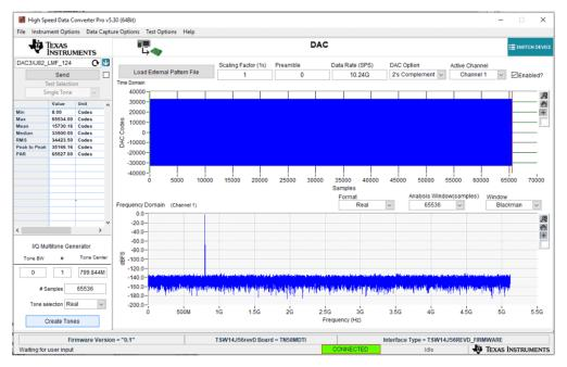
Figure 3-39. DAC Test Pattern Display
