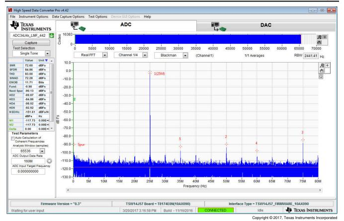
Figure 7-4. ADC34J45 Operating in 14-Bit Mode at 160 Msps with 25-MHz Input Signal
