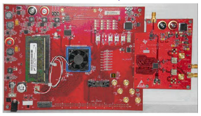
Figure 5-1. TSW1400 EVM Interfacing to a DAC EVM
