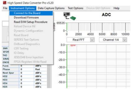
Figure 2-5. Connecting GUI to EVM
