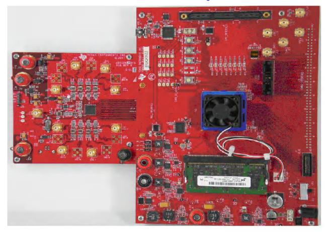
Figure 4-1. TSW1400EVM interfacing to an ADS5281 EVM
