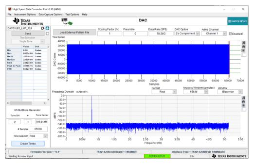
Figure 5-4. TSW1400 Output Data to DAC EVM
