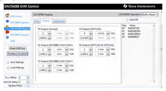
Figure 5-6. CDCM7005 Tab on DAC5688 GUI
