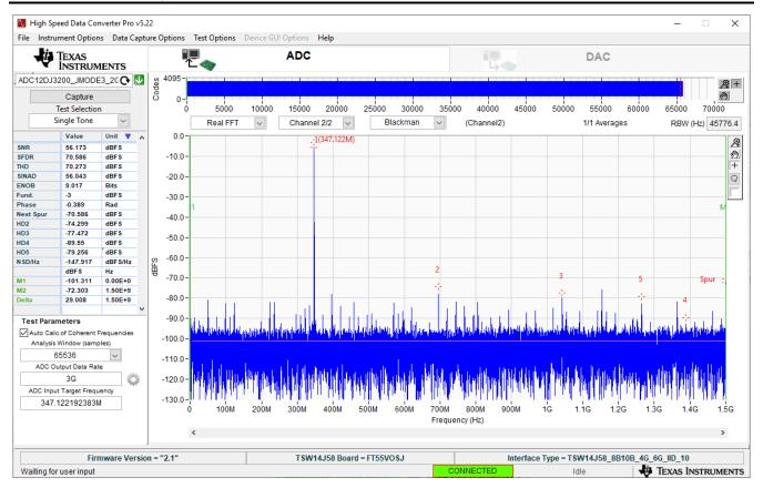
Figure 6-4. ADC12DJ3200 Operating in JMODE3 at 3 Gsps with 347-MHz Input Signal
