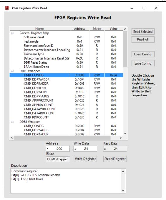
Figure 3-8. FPGA Registers Write Read Window
