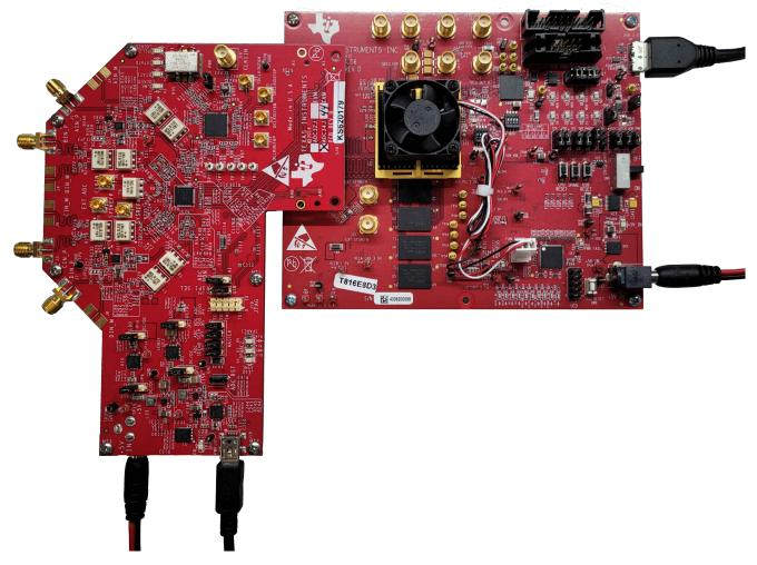
Figure 8-2. TSW14J56 EVM connected to an ADC34J45 EVM
