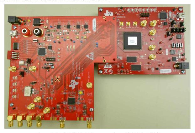
Figure 9-1. TSW14J50 EVM Connected to an ADS42JB69 EVM
