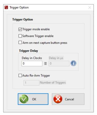
Figure 3-13. Slave Trigger Setup
