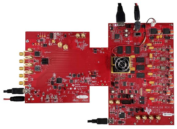
Figure 6-2. TSW14J58 EVM connected to an ADC12DJ3200 EVM
