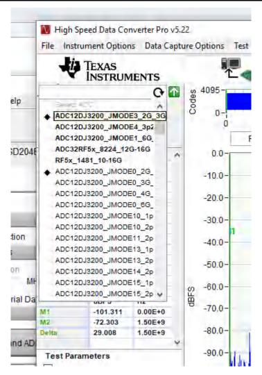
Figure 6-3. Select ADC12DJ3200\_JMODE3\_2G\_3G in the HSDC Pro GUI Program
