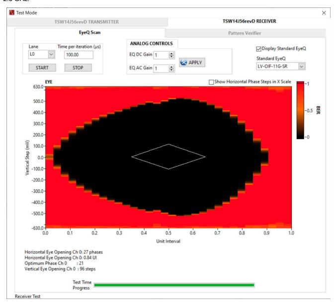
Figure 3-5. Example Eye Diagram Plot
