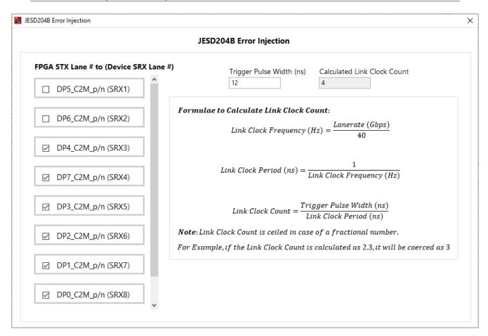
Figure 3-7. JESD204B Error Injection Window
