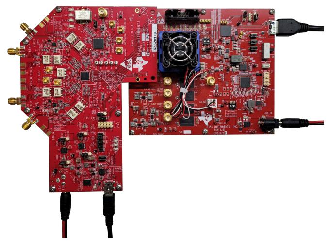
Figure 7-2. TSW14J57 EVM connected to an ADC34J45 EVM
