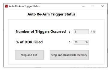
Figure 3-11. Auto Re-Arm Trigger Status Window
