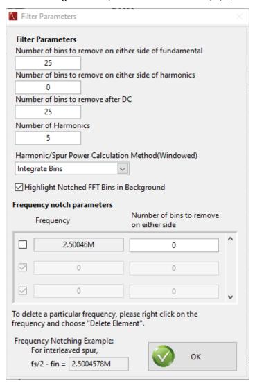
Figure 3-18. Notch Frequency Bin Removal
