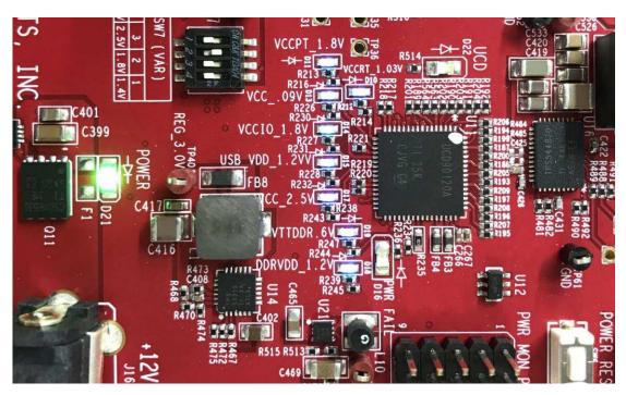
Figure 3. Power Indicator LEDs
