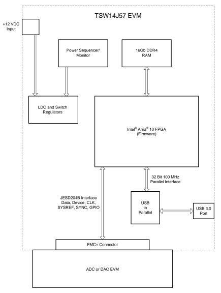
Figure 2. TSW14J57 EVM Block Diagram
