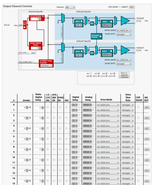
Figure 13. GUI: Outputs
