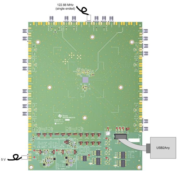
Figure 1. LMK04616 EVM Quick Start Connection
