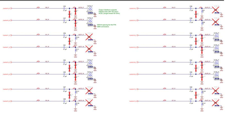
CLOCK OUTPUT (OUT#\_P, OUT#\_N) LAYOUT REQUIREMENTS: \*\*\*\* CONTROLLED IMFEDANCE \*\*\*\* - Route as 50-ont (+-5% tol.) controlled-impedance single-ended RF traces from DUT pin to SMA pim - Place component pads directly on RF traces (no stubs), match 50-ohm trace will MEMSter pad (30 mils wide), and use 50-ohm Zo via structures. \*\*\* LENGTH / SKEW MATCHING \*\*\*
