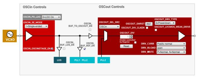
Figure 8. GUI: OSCin and OSCout
