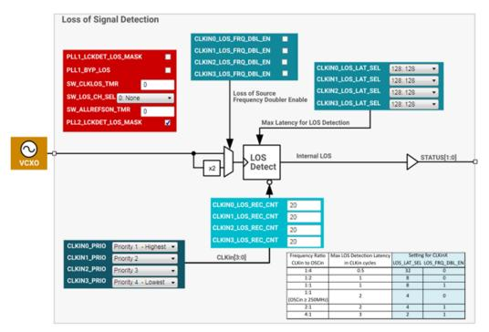
Figure 9. GUI: LOS Control
