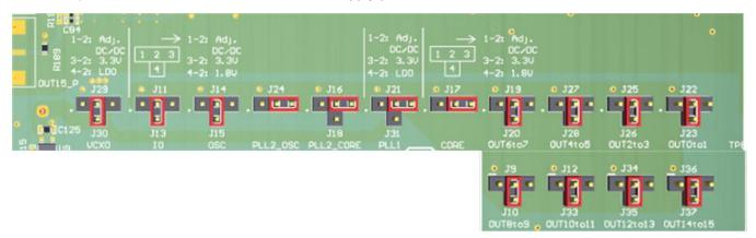
Figure 17. Power Distribution Jumpers
