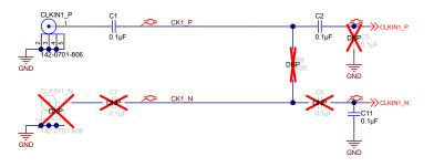
By default, CLKIN1 SMA is DC coupled to the 51 Ohm, then AC coupled to CLKIN1 input CLKIN1 is single-ended by default (negative input is connected to 0.1uA)
