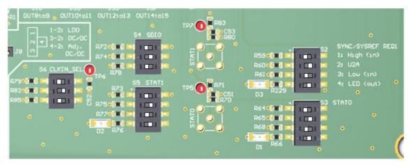
Figure 21. Default Dip Switch Setting
