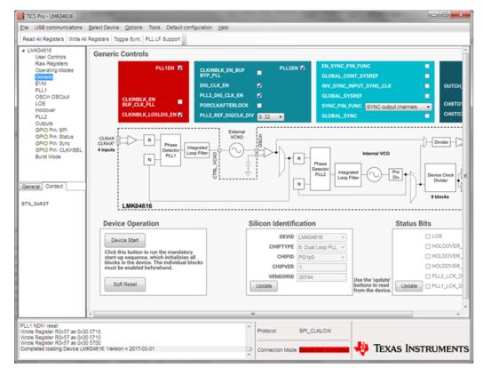
Figure 5. TICS Pro With LMK04616 GUI Loaded
