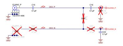
By default, CLKIN3 SMA is DC coupled to the 100 Ohm, then AC coupled to CLKIN3 input
