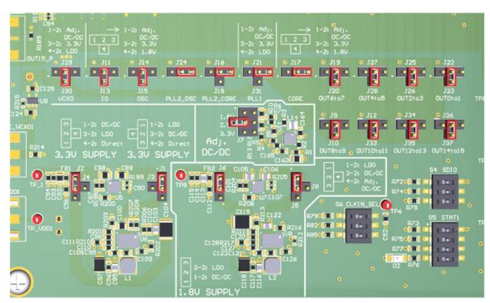
Figure 16. Default Power Supply Connection
