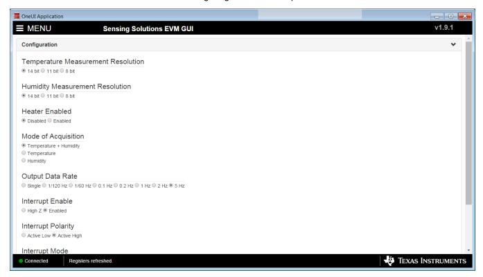
Figure 33. HDC2010 GUI Configuration Page
