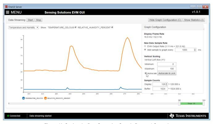
Figure 40. Setting the Data Streaming Sample Rate to 1 Second
