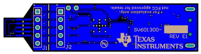
Figure 55. Bottom Layer Routing
