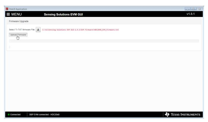
Figure 51. Upload Firmware Button on Firmware Upload Page
