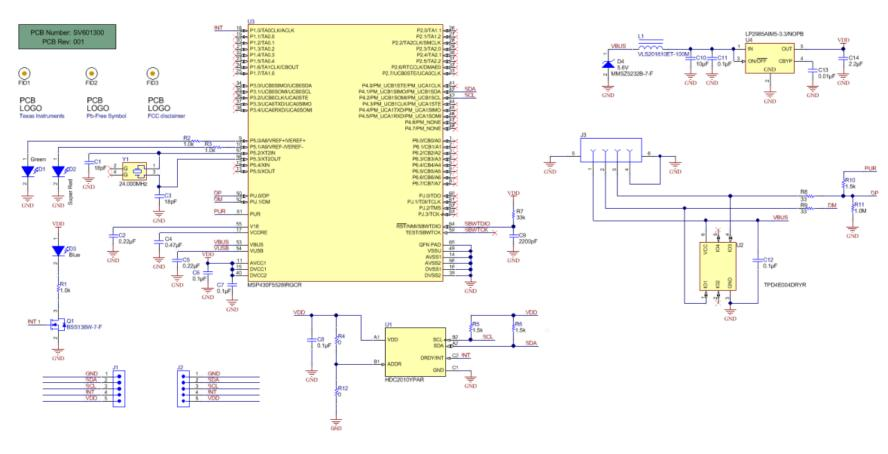
Figure 56. HDC2010EVM Schematic
