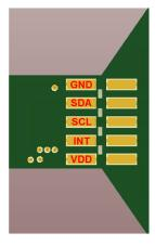
Figure 14. HDC2010EVM: Pads for I2C and Supply of the Smaller Sensor Module
