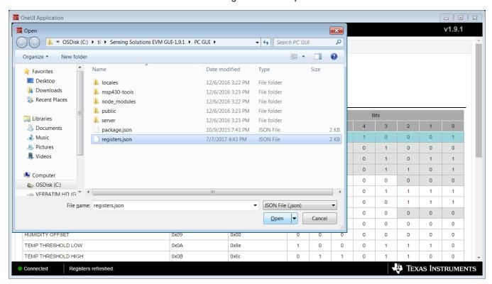
Figure 32. Selecting Previously Save Register Value JSON File
