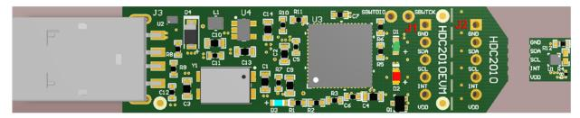
Figure 13. HDC2010EVM: PC Interface and Smaller Sensor Module
