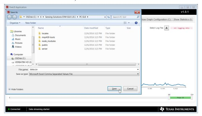
Figure 38. Selecting the Log File for Data Streaming
