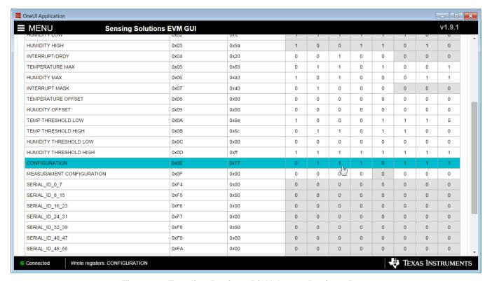
Figure 26. Toggling Register Bit Value on Register Page
