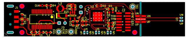
Figure 8. Top Assembly Layer as Viewed From Top of Board
