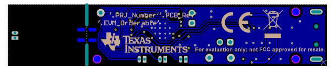
Figure 12. Bottom Assembly Layer as Viewed From the Bottom
