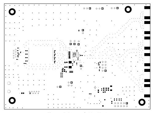
Figure 15. Bottom Solder Mask
