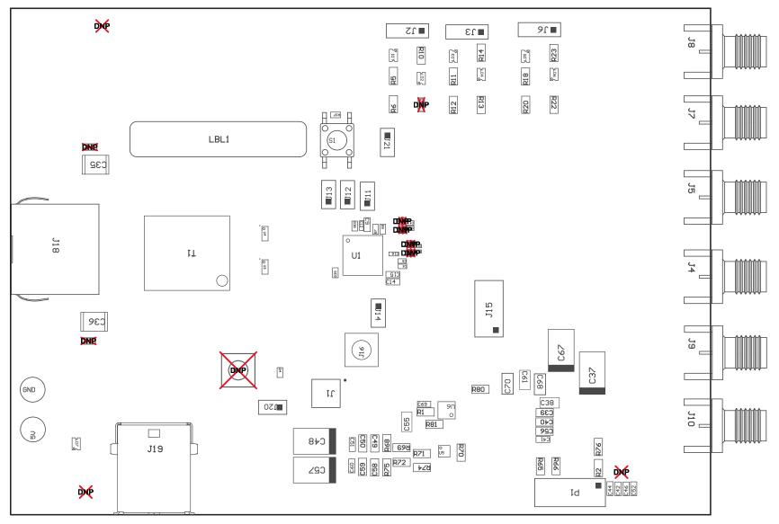
Figure 16. Board Assembly Top
