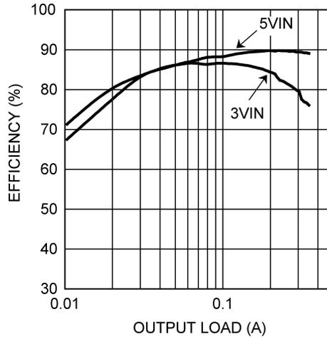
**Figure 3. LM2735Y  $\eta$  vs Load Current,  $V_o = 12V$**
