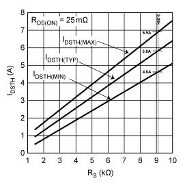
Figure 4.  $R_s vs I_{DSTH}$  for  $R_{DS(ON)} = 25 m\Omega$
