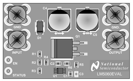
Figure 8. Component Placement
