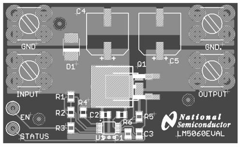
Figure 9. Evaluation Board, Top Side (Component)
