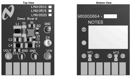
Figure 1. LMR10510/LMR10515/LMR10520 Demo Board
