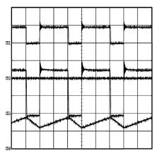
Figure 6. V<sub>IN</sub> = 18 V, I<sub>OUT</sub> = 3 A Illustrating Buck Operation CH1: V<sub>SW</sub> = 20V/div; CH2: Q1 = 20V/div; CH3: Q2 = 10V/div; CH4: I<sub>L</sub> = 2A/div
