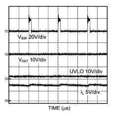
Figure 3. Short Circuit Current
