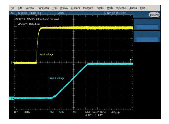
FIGURE 11. Start-up waveforms Vin=60V, lout=1.5A
