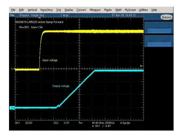
FIGURE 10. Start-up waveforms Vin=36V, lout=1.5A
