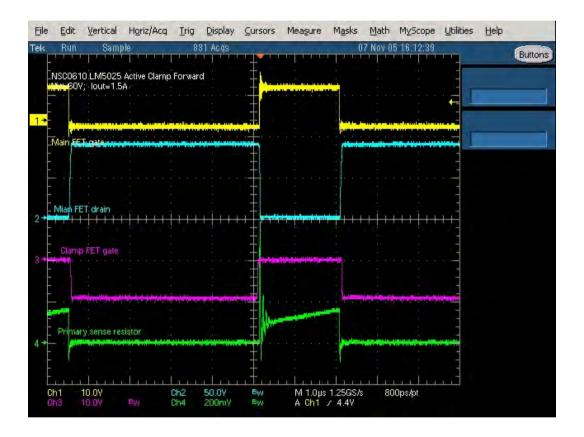
FIGURE 13. Switching waveforms Vin=60V, lout=1.5A
