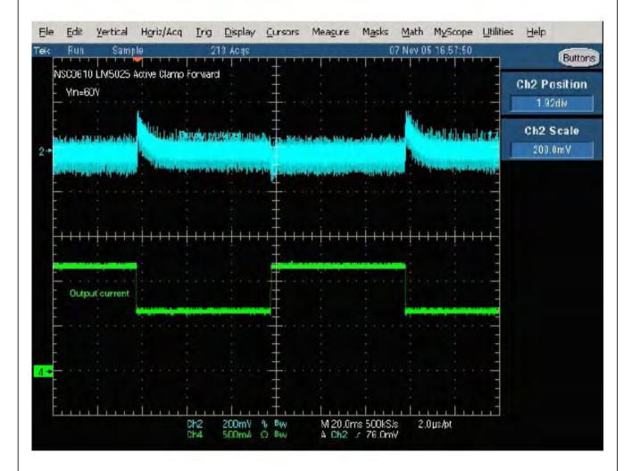
FIGURE 9. Transient response, Vin = 36V with a step response of .5A to 1A
