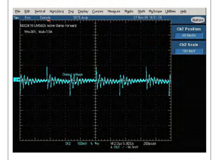
FIGURE 8. Output ripple, Vin = 36V with full load
