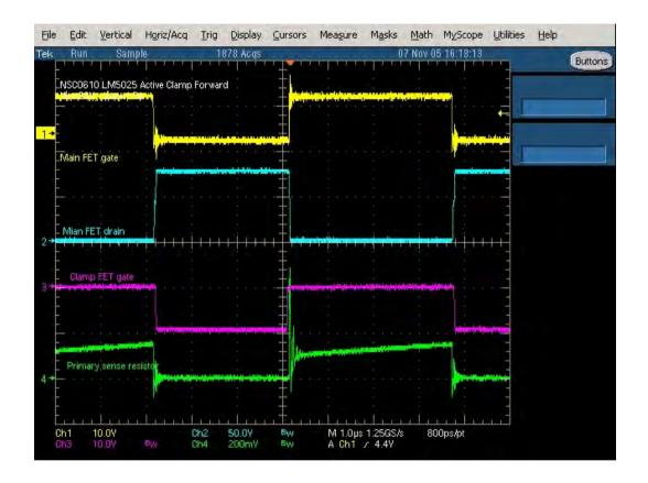
FIGURE 12. Switching waveforms Vin=36V, lout=1.5A
