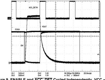
Figure 9. ENABLE and ACC\_DET Cycled Independently, VCC = 5.3V
