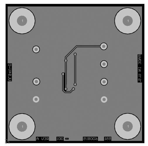
Figure 11. PCB Bottom Layer
