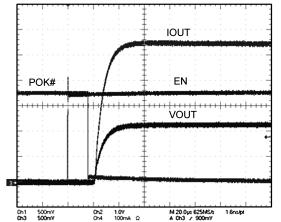
Figure 7. ENABLE Turn On Into An Overload Condition ( $4\Omega$  Resisitve Load), VCC = 5.3V
