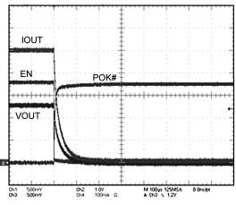
Figure 5. ENABLE Turn Off, VCC = 2.8V, IOUT = 0.5A (Resistive Load)
