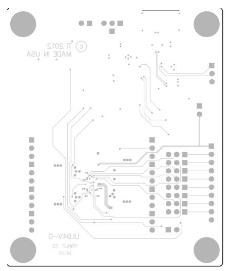
Figure 10. LM10507 Board Inner Layer 4
