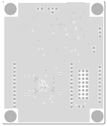
Figure 8. LM10507 Board Inner Layer 2
