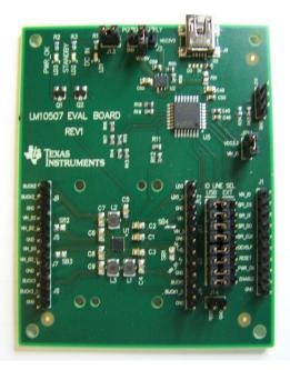
Figure 1. LM10507 Evaluation Board
