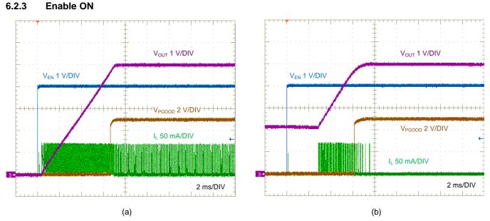
Figure 9. Enable ON at  $V_{IN}$  = 24 V: (a)  $I_{OUT}$  = 12.5 mA, (b) No Load, 2-V Output Pre-bias
