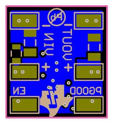
Figure 17. Bottom Copper (Bottom View)
