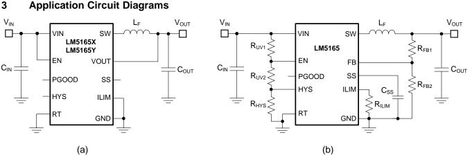
Figure 1. LM5165 PFM-controlled Buck Converter Schematics, (a) Fixed Output of 3.3 V or 5 V, (b) Adjustable Output with Soft-start, Current Limit and Input UVLO Components
