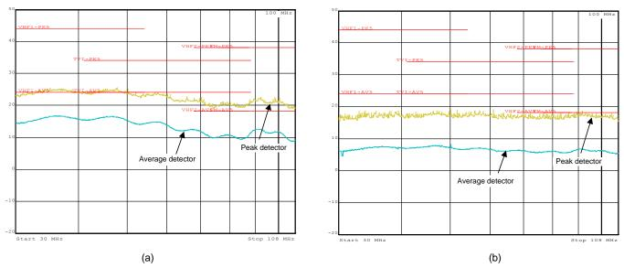
Figure 12. CISPR 25 Class 5 Conducted Emissions Plot, 30 MHz to 108 MHz, V<sub>IN</sub> = 13.5 V, I<sub>OUT</sub> = 25 mA: (a) Unfiltered, (b) Filtered
