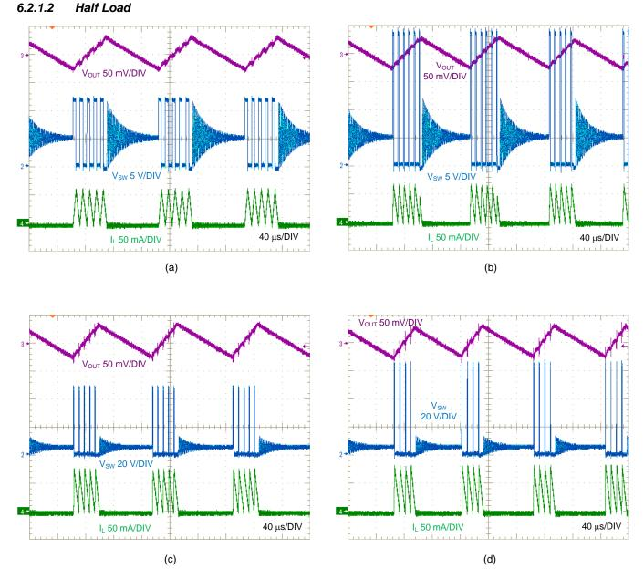
Figure 6. SW Node,  $V_{out}$  and  $I_L$  Waveforms at  $I_{out}$  = 12.5 mA: (a)  $V_{IN}$  = 12 V, (b)  $V_{IN}$  = 24 V, (c)  $V_{IN}$  = 36 V, (d)  $V_{IN}$  = 65 V
