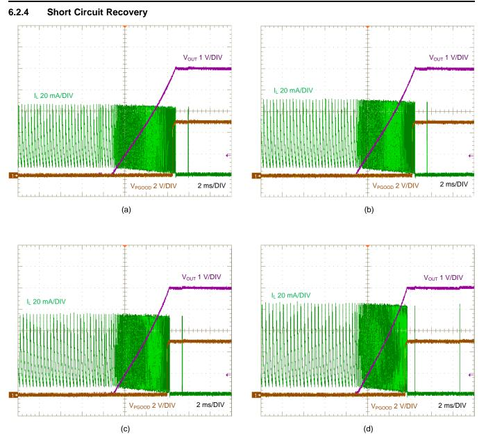
Figure 10. Short Circuit Recovery into No Load: (a)  $V_{IN} = 12 V$ , (b)  $V_{IN} = 24 V$ , (c)  $V_{IN} = 36 V$ , (d)  $V_{IN} = 65 V$
