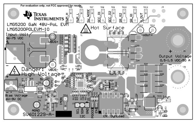
Figure 11. LMG5200POLEVM-10 Top Layer and Components
