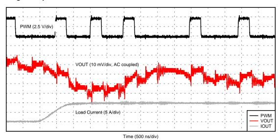
Figure 9. Typical Switching Waveforms
