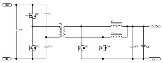
Figure 1. Half-Bridge with Current-Doubler Rectifier
