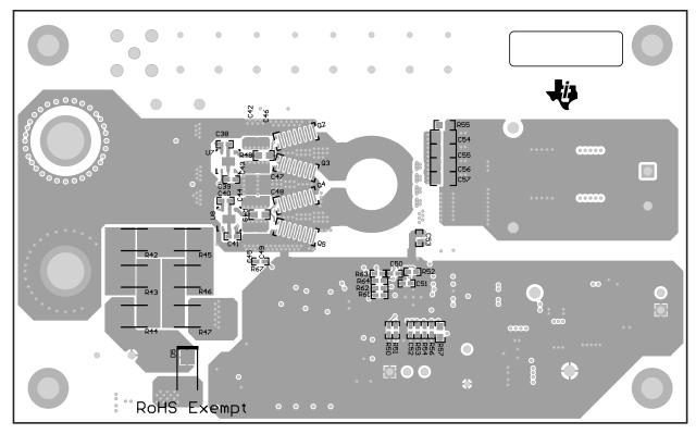
Figure 12. LMG5200POLEVM-10 Bottom Layer and Components
