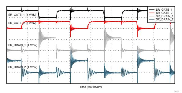
Figure 8. Secondary-Side Switching Waveforms
