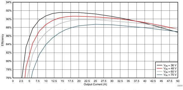
Figure 6. LMG5200POLEVM-10 Efficiency vs Input Voltage
