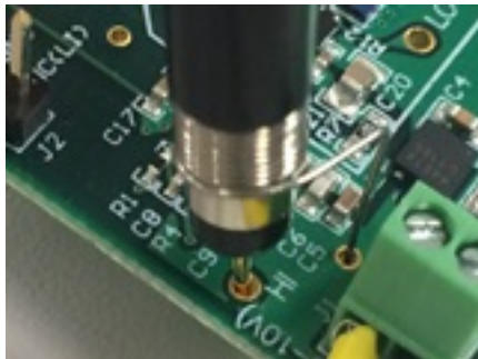
Figure 4. HI Test Point (TP8)
