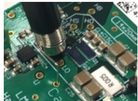
Figure 9. LO Test Point (TP11)
