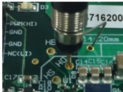
Figure 8. HO Test Point (TP3)
