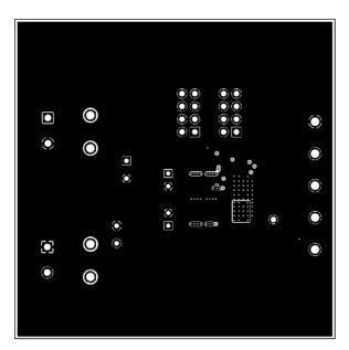
Figure 9. Layer 2 Copper (Top View)
