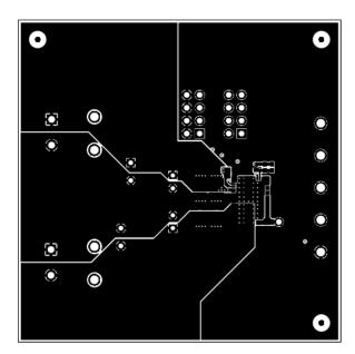
Figure 8. Topside Copper (Top View)
