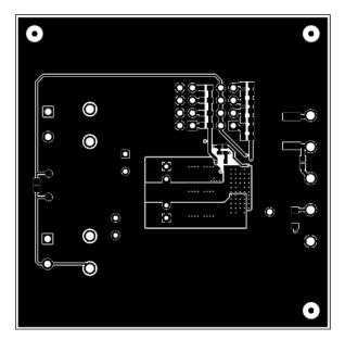
Figure 11. Bottom-Side Copper (Top View)
