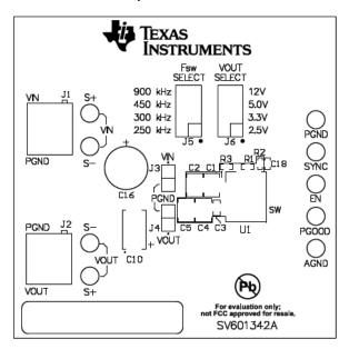
Figure 7. Topside Component Layout (Top View)
