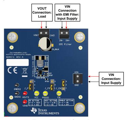
Figure 1. EVM Board Connections
