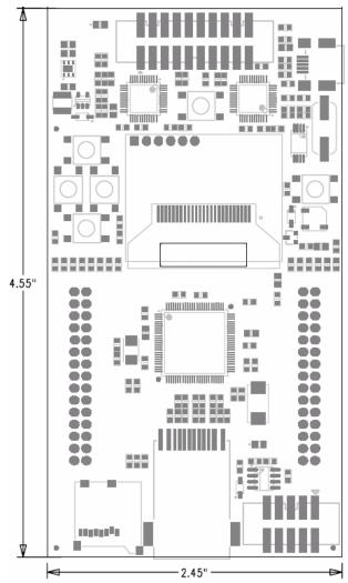
Figure B-3. LM3S2110 CAN Device Board Dimensions
