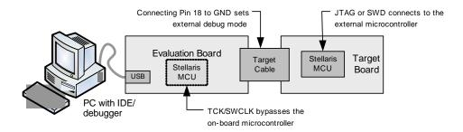
The debug interface operates in either serial-wire debug (SWD) or full JTAG mode, depending on the configuration in the debugger IDE.
