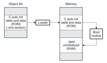
Figure 6-6. Autoinitialization at Run Time
