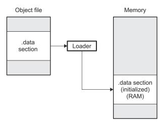
Figure 6-7. Initialization at Load Time
