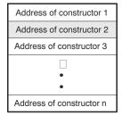
Figure 6-10. Format of Initialization Records in the .pinit Section
