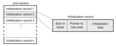
Figure 6-9. Format of Initialization Records in the .cinit Section
