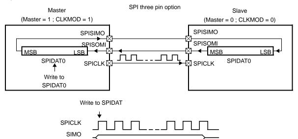
Data written to the shift register (SPIDAT0) initiates data transmission on the SPISIMO pin, most significant bit (MSB) first. Simultaneously, received data is shifted through the SPISOMI pin into the least significant bit (LSB) of the SPIDAT0 register. When the selected number of bits has been transmitted, the data is transferred to the SPIBUF register for the CPU to read. Data is stored right-justified in SPIBUF.
