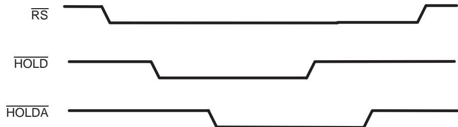
Figure 4–9. \overline{\text{HOLD}} Deasserted Before Reset Deasserted
