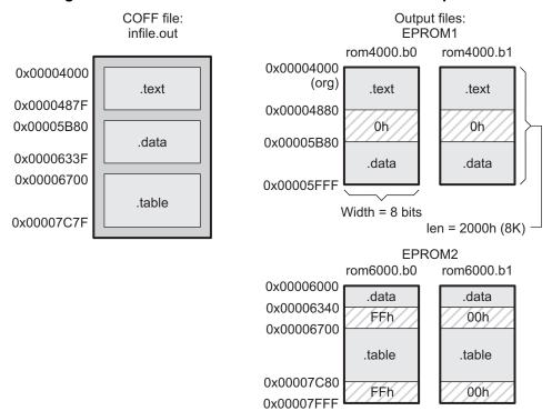
The map file (specified with the --map option) is advantageous when you use the ROMS directive with multiple ranges. The map file shows each range, its parameters, names of associated output files, and a list of contents (section names and fill values) broken down by address. Example 11-2 is a segment of the map file resulting from the example in Example 11-1.
