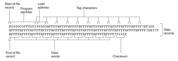
If any data fields appear before the first address, the first field is assigned address 0000h. Address fields may be expressed but not required for any data byte. The checksum field, preceded by the tag character 7, is the 2s complement of the sum of the 8-bit ASCII values of characters, beginning with the first tag character and ending with the checksum tag character (7 or 8). The end-of-file record is a colon (:).
