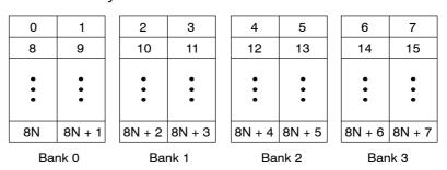
For devices that have more than one memory block (see Figure 5–23), an access to bank 0 in one block does not interfere with an access to bank 0 in another memory block, and no pipeline stall occurs.
