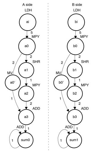
Figure 5–20. Dependency Graph of Live-Too-Long Code (Split-Join Path Resolved)
