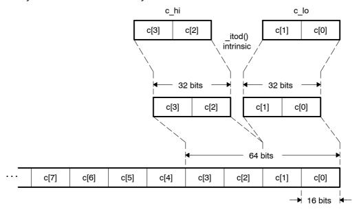
This code now efficiently reads and writes large amounts of data. The next step is to find a method to quickly add them. The \_add2() intrinsic provides just that: It adds corresponding packed elements in two different words, producing two packed sums. It provides exactly what is needed, a vector addition. Figure 6–13 illustrates.
