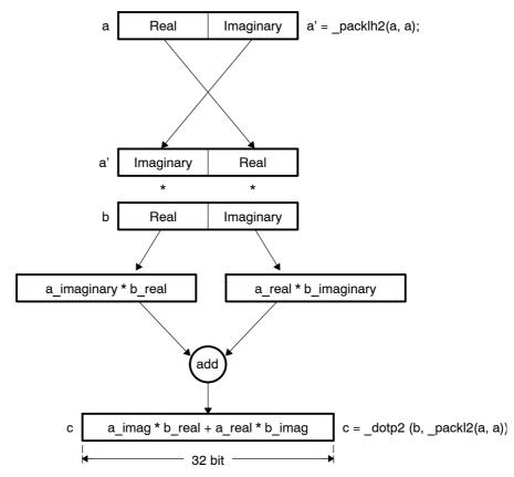
Figure 6-20. \_packlh2 and \_dotp2 Working Together.
