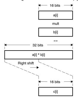
Notice that the values are still loaded and stored as 16-bit quantities. Therefore, you should use the same basic flow as the vector sum. Example 6–7 shows this starting point. Figure 6–11 and Figure 6–12 also apply to this example to illustrate how data is being accessed.
