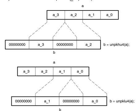
Figure 6-6. Graphical Representation of 8-Bit Unpacks (unpkXu4)
