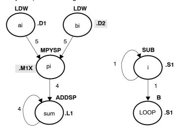
Figure 5-4. Dependency Graph of Floating-Point Dot Product With Parallel Assembly
