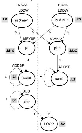
Figure 5–10. Dependency Graph of Floating-Point Dot Product With LDDW (Showing Functional Units)
