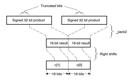
Whether or not the 16-bit shift version is used, consider the vector multiply to be fully optimized from a packed data processing standpoint. It can be further optimized using the more general techniques such as loop-unrolling and software pipelining that are discussed in Chapter 2.
