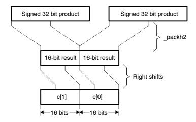
Figure 6–17. Fine Tuning Vector Multiply (shift < 16)
