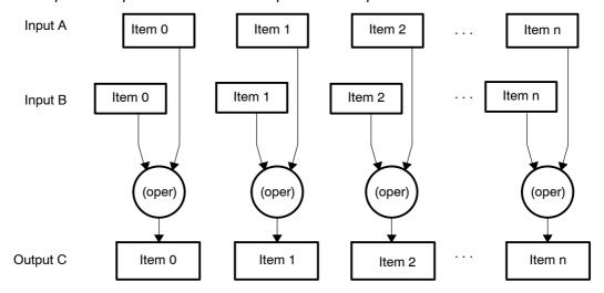
Although pure vector algorithms exist, most applications do not consist purely of vector operations as simple as the one shown in Figure 6–8. More commonly, an algorithm will have portions, which behave as a vector algorithm, and portions which do not. These portions of the code are addressed by other packed-data processing techniques.
