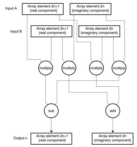
Figure 6–10. Graphical Representation of a Single Iteration of Vector Complex Multiply.
