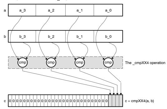
Figure 6-22. Graphical Illustration of cmpXX4 Intrinsics
