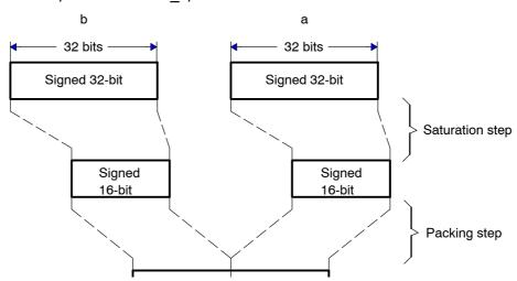
Figure 6-4. Graphical Representation of spack2
