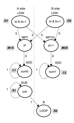
Example 5–21. Linear Assembly for Fixed-Point Dot Product Inner Loop (With Conditional SUB Instruction)
