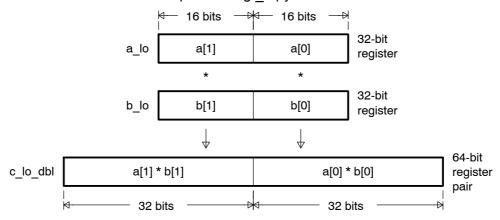
Once the 32-bit products are obtained, use standard 32-bit shifts to shift these to their final precision. However, this will leave the results in two separate 32-bit registers.
