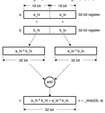
This operation exactly maps to the operation the dot product kernel performs. The modified version of the kernel absorbs two of the four ADDs into \_dotp intrinsics. The result is shown as Example 6–11. Notice that the variable c has been eliminated by summing the results of the \_dotp intrinsic directly.
