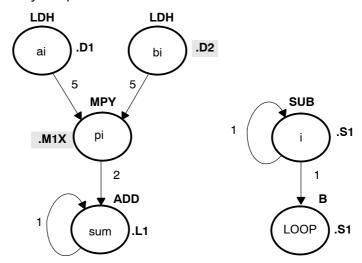
Figure 5-3. Dependency Graph of Fixed-Point Dot Product with Parallel Assembly
