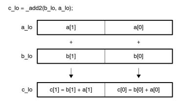
So, putting in \_add2() to perform the additions provides the complete code shown in Example 6–6.
