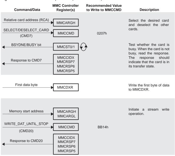
Figure 2–7. Stream Write Operation (MMC Protocol)
