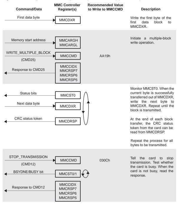
Figure 2–6. Multiple-Block Write Operation (MMC Protocol) (Continued)
