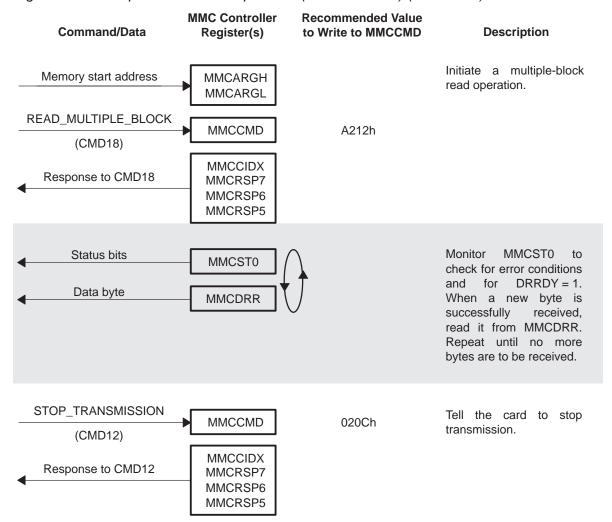
Figure 2–3. Multiple-Block Read Operation (MMC Protocol) (Continued)
