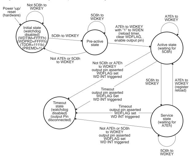
Figure 2–2. Watchdog Timer Operation State Diagram
