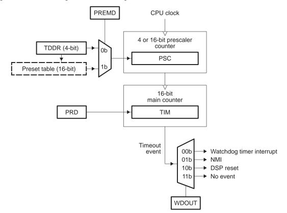
Figure 2–1. Watchdog Timer Block Diagram
