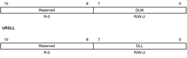
Legend: R = Read; W = Write; -n - Value after reset; -U = Value unchanged by reset
