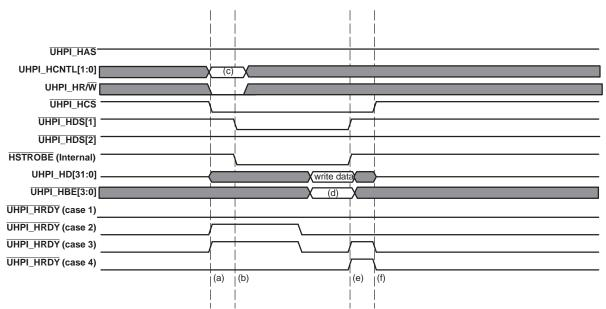
Figure 8. Multiplexed Host Address/Data Fullword Write (without UHPI\_HAS)
