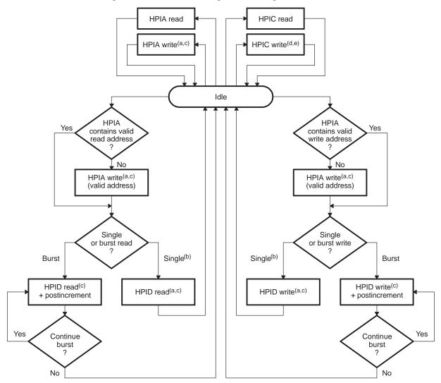
Figure 17. UHPI State Diagram for Single HPIA Mode
