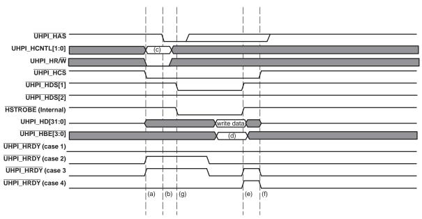
Figure 9. Multiplexed Host Address/Data, Fullword Write (using UHPI\_HAS)
