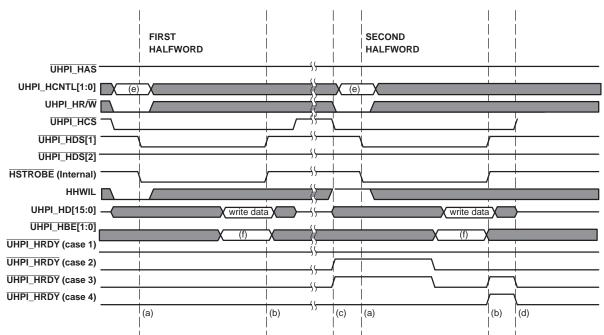
Figure 12. Multiplexed Host Address/Data Dual Halfword Write (without UHPI\_HAS)
