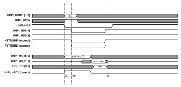
Figure 14. Non-Multiplexed Host Address/Data Fullword Read
