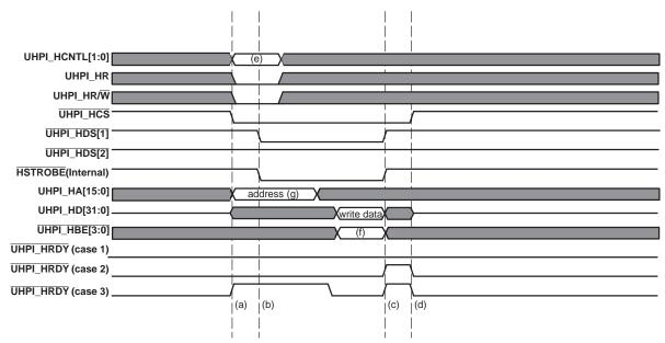
Figure 15. Non-Multiplexed Host Address/Data Fullword Write
