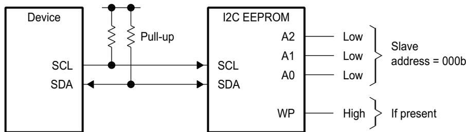
Some I2C EEPROMs have a write-protect (WP) feature that prevents unauthorized writes to memory. This feature is not needed for boot loading purposes because the DSP only reads data from the I2C EEPROMs. The write protect feature can be enabled or disabled without impacting bootloader operation.
