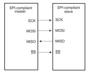
Figure 41. Typical SPI Interface
