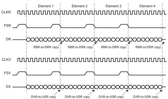
Figure 21. Maximum Frame Frequency Operation With 8-Bit Data
