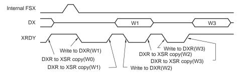
(d) XMCM = 3h, RPABLK = 0, XPABLK = x, RCERE0 = 0000 0008h, XCERE0 = 0000 000Ah: Receive channels: 1 and 3 enabled; transmit channels: 1 and 3 enabled, but only 3 unmasked
