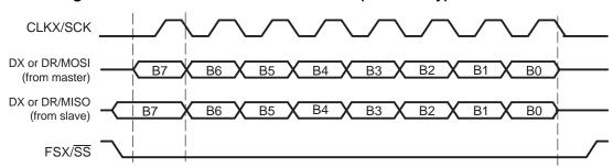
Figure 43. SPI Transfer With CLKSTP = 3h (clock delay) and CLKXP = 0
