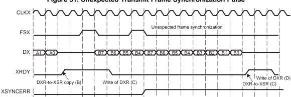
Figure 31. Unexpected Transmit Frame Synchronization Pulse
