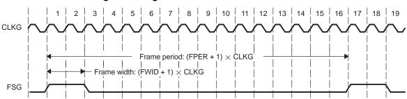
Figure 9. Programmable Frame Period and Width
