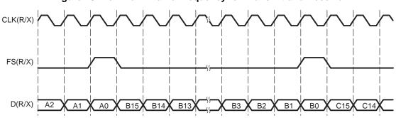
Figure 18. Maximum Frame Frequency for Transmit and Receive
