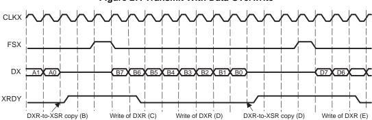
Figure 27. Transmit With Data Overwrite
