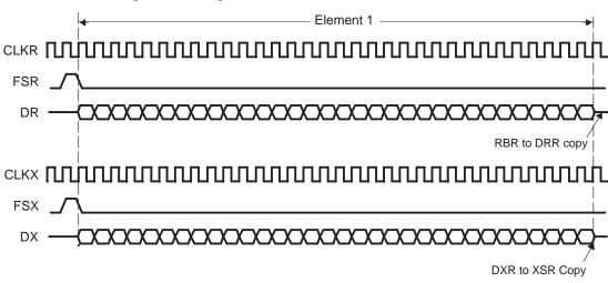
Figure 12. Single-Phase Frame of One 32-Bit Element
