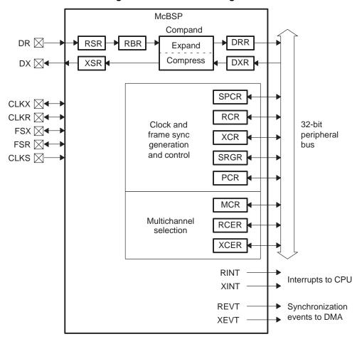
Figure 1. McBSP Block Diagram
