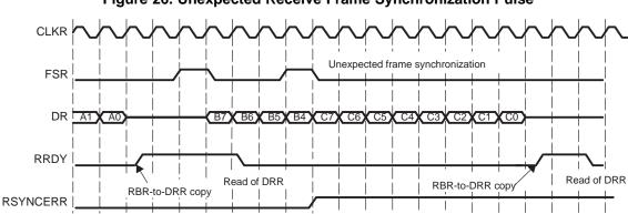
Figure 26. Unexpected Receive Frame Synchronization Pulse
