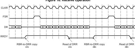
Figure 16. Receive Operation
