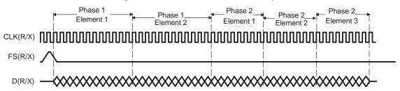
Table 7. RCR/XCR Fields Controlling Elements per Frame and Bits per Element
