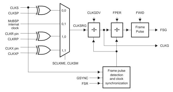
Figure 5. Sample Rate Generator Block Diagram
