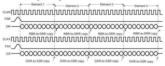
Figure 11. Single-Phase Frame of Four 8-Bit Elements
