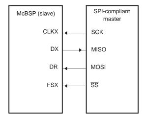
Figure 47. McBSP as an SPI Slave
