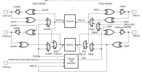
Figure 2. Clock and Frame Generation
