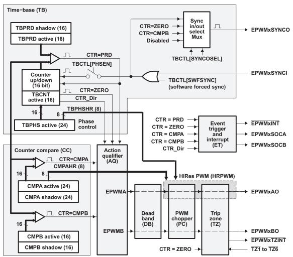
Figure 4. HRPWM System Interface
