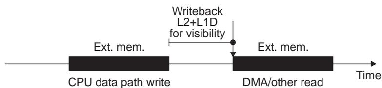
**Figure A-4. L2 SRAM/External Memory: CPU Write (Data), CPU Read (Code)**
