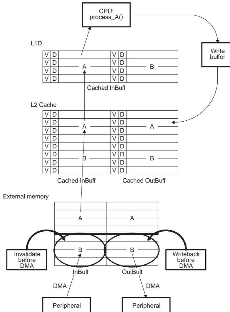
The chip support library (CSL) provides a set of routines that allow the required cache coherence operations to be initiated. The start address of the buffer in external memory and the number of bytes need to be specified:
