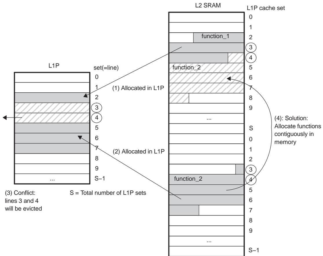
**Note:** With code generation tools 5.0 (CCS 3.0) and later, the GROUP directive **must** be used to force a specific link order.
