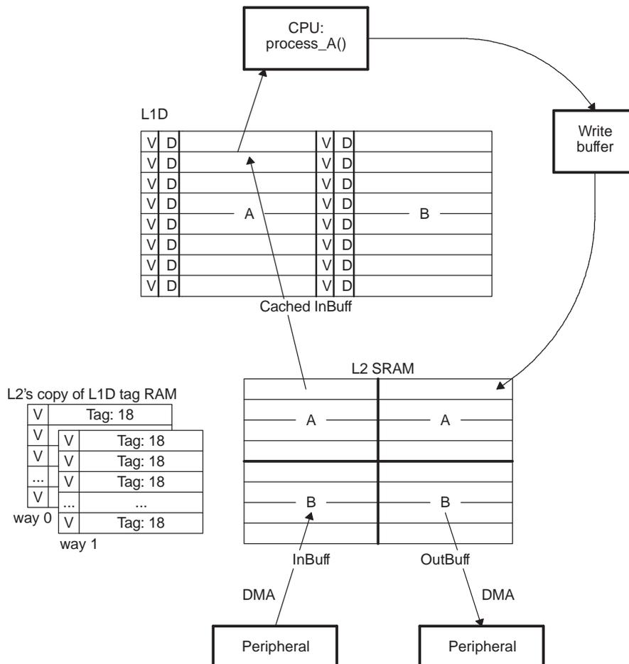
**Example 2-3. L2 SRAM DMA Double Buffering Code**
