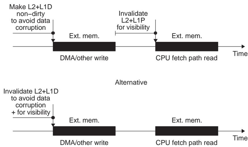
**Figure A-3. External Memory: CPU Write, DMA Read (Data)**
