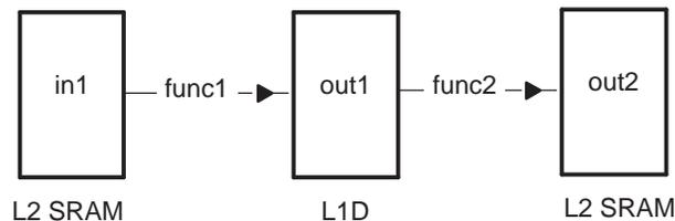
Consider [Example 3-2](#), a 4-channel filter system consisting of a FIR filter followed by a dot product. The FIR filter in the first iteration allocates `in[ ]` and `h[ ]` in L1D and writes `out[ ]` to L2 SRAM. Subsequently, `out[ ]` and `w[ ]` are allocated in L1D by the dotprod routine. For the next iteration, the FIR routine writes its results to L1D, rather L2 SRAM, and the function dotprod does not incur any read misses.
