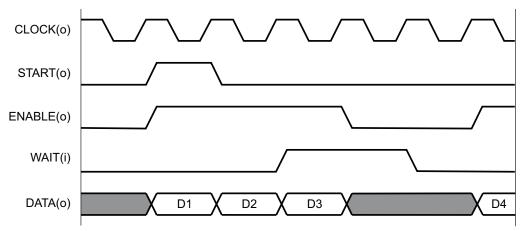
Figure 10. Signal Timing for uPP Channel in Transmit Mode with Single Data Rate
