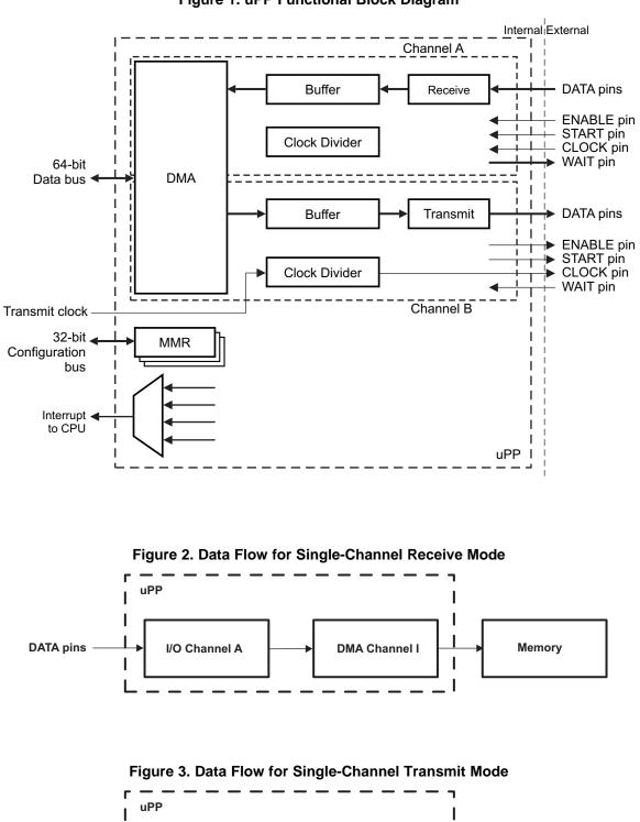
Figure 1. uPP Functional Block Diagram
