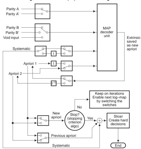
Figure 4. Standalone (SA) Mode Block Diagram
