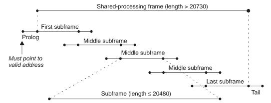
Figure 97. Shared Processing Subframe Segmentation (Example with 5 Subframes)
