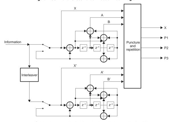
Figure 1. 3GPP and IS2000 Turbo-Encoder Block Diagram
