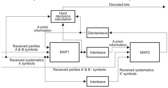
Figure 2. 3GPP and IS2000 Turbo-Decoder Block Diagram
