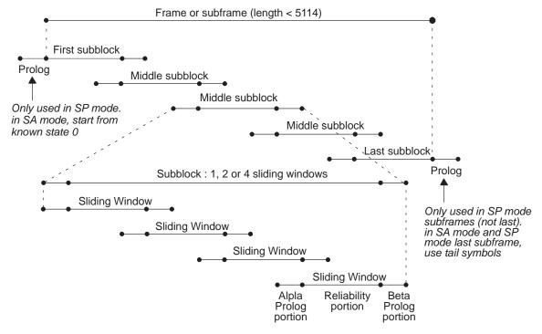
Figure 96 show diagrams for the sliding windows for both alpha and beta. Each sliding window consists of a reliability section and a prolog section. The size of the reliability section can range from 40 to 128 and the size of the prolog section can range from 4 to 48 in the TCP2. The alpha sliding window starts at the left and goes right (forward order) and the beta sliding window starts at the right and goes left (reverse order). See Table 40 for the number of sub-blocks and sliding windows.
