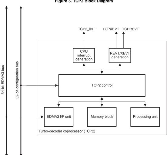
Figure 3. TCP2 Block Diagram
