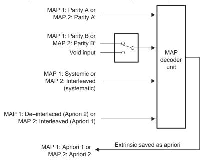
Figure 19. TCP2 Shared Processing Block Diagram
