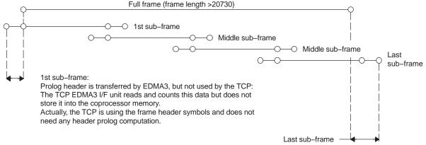
A full sub–frame including the header and tail prolog is transferred by EDMA3 but the totality is not used by the TCP.
