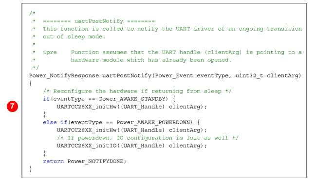
If the device is powered down, the IO configuration is also lost, so UARTCC26XX\_initIO() is called.
