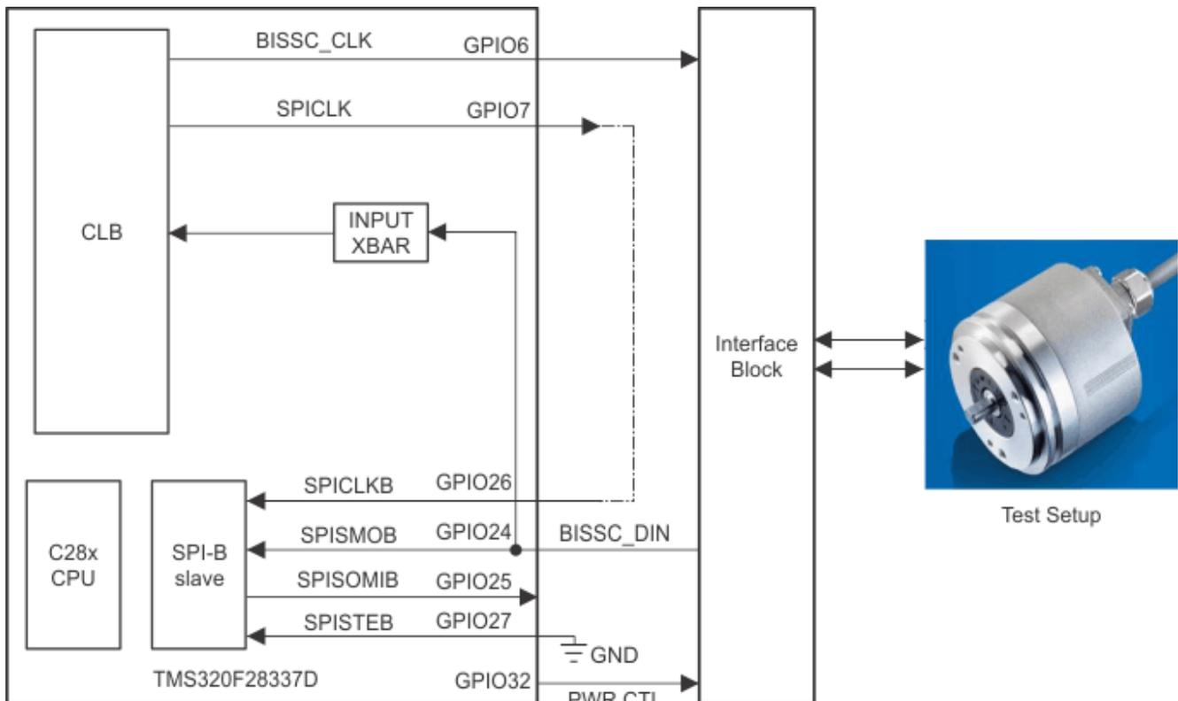
Figure 1-3. BiSS-C Implementation Diagram Inside TMS320F28379D
