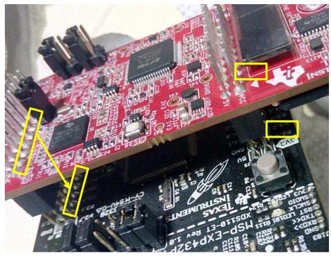
Figure 23. C5545 BoosterPack Connected With MSP432P401R LaunchPad
