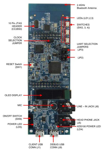
Figure 2. C5545 BoosterPack Top View
