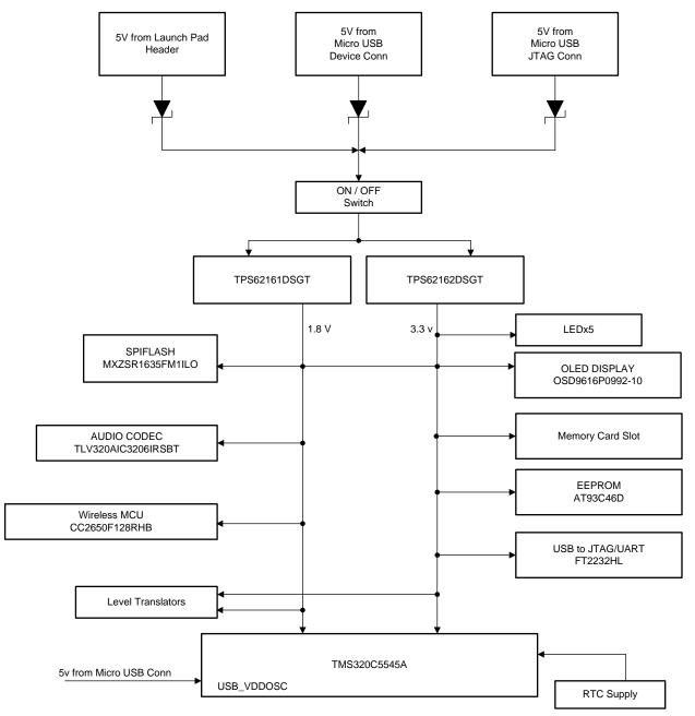
Figure 31. Power Distribution Diagram
