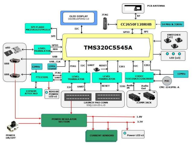
Figure 1. C5545 BoosterPack Functional Block Diagram
