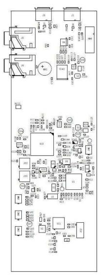
Figure 26. C5545 BoosterPack Board Assembly Layout - Top View
