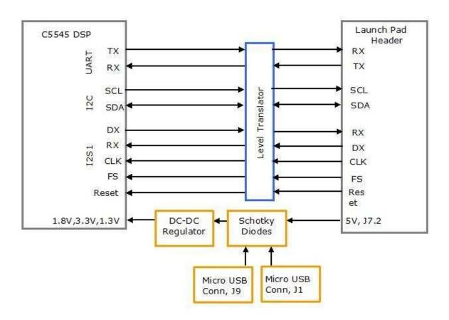
Figure 20. Connection Between C5545 and LaunchPad
