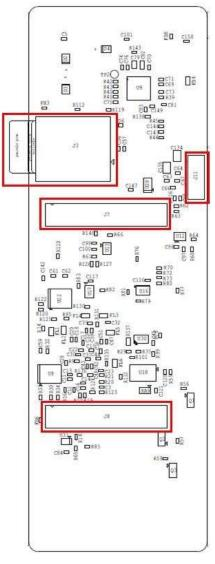
Figure 29. Connectors on C5545 BoosterPack - Bottom
