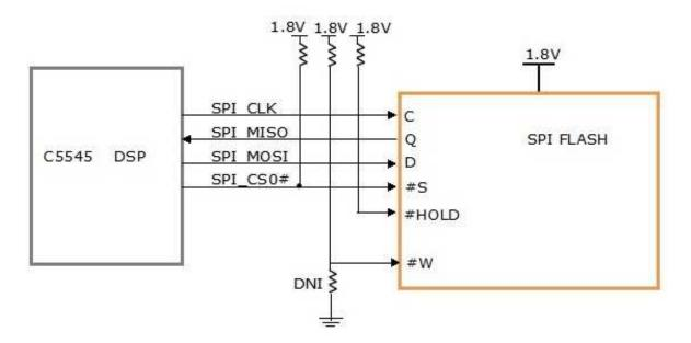
Figure 7. SPI FLASH Interface
