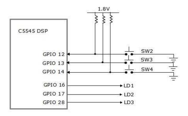
Figure 8. Switch and LED Connection
