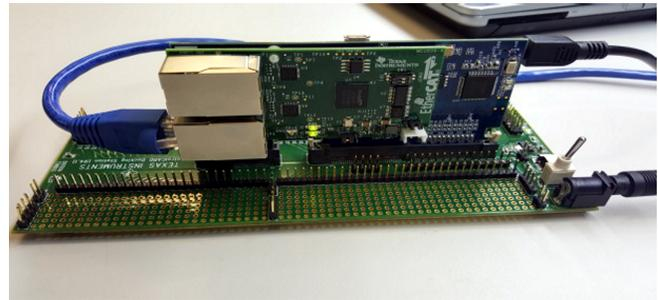
**Figure 2. TMDSECATCNCD379D Hardware Kit (5V Supply)**
