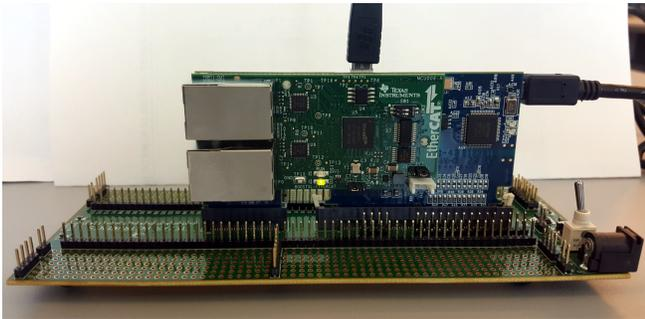
**Figure 1. TMDSECATCNCD379D Hardware Kit (Micro USB)**
