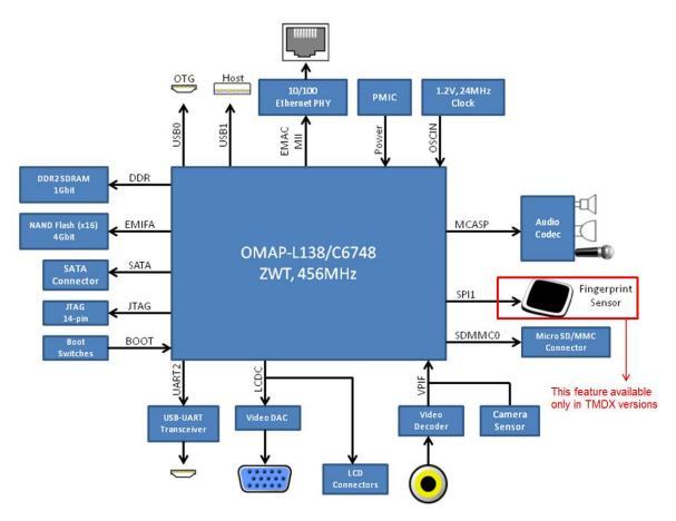
Figure 1. LCDK Block Diagram
