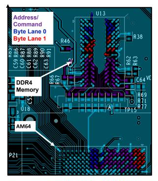
Figure 6-1. DDR4 Address and Data Top Layer
