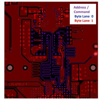
Figure 6-3. DDR4 Address on Bottom Layer
