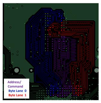
Figure 6-4. DDR4 Address and Data Sig2 Layer
