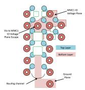
Figure 7-2. Alternate AM64 GP EVM Output Capacitor Placement for CAP\_VDDSHV\_MMC1
