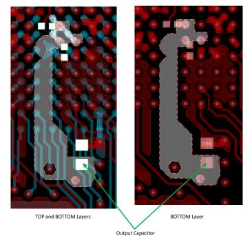
Figure 7-1. AM64 GP EVM Output Capacitor Placement for CAP\_VDDSHV\_MMC1
