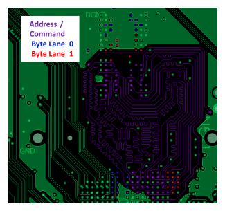
Figure 6-2. DDR4 Address on Sig1 Layer
