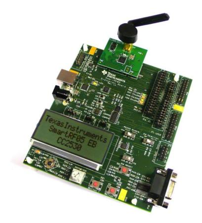
Figure 7 - SmartRF05EB with EM connected
