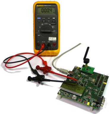
Figure 14 - Current measurement set-up
