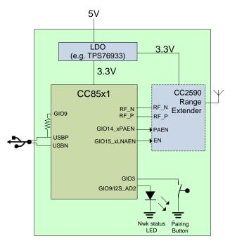
Figure 3 - Application block diagram for USB device
