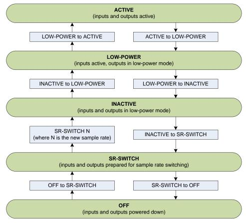
Figure 49 - Audio device state transitions
