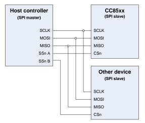
Figure 7 - SPI slave interface
