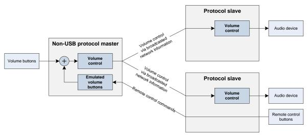
Figure 50 – A protocol slave using remote control commands to control volume for all slaves
