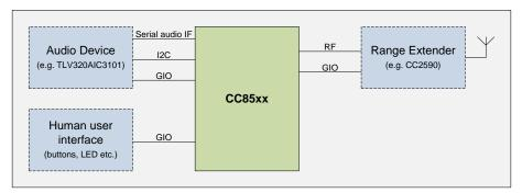
Figure 41 - Autonomously operated system
