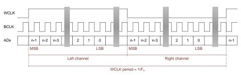
Figure 15 - Left-justified interface format
