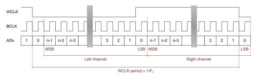
Figure 14 - I<sup>2</sup>S interface format
