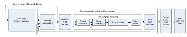
Figure 32 – SLAC encoding (16-bit)
