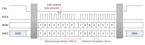
Figure 8 - SPI interface behavior
