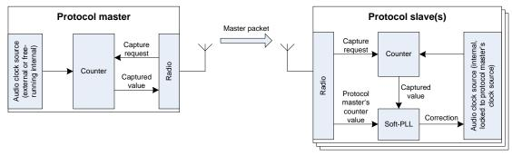
Figure 27 - Clock distribution overview for non-USB system
