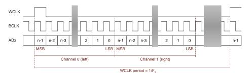
Figure 17 - DSP interface format (showing 2 first of 8 possible channels)
