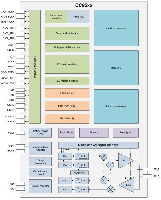
Figure 6 - Block diagram
