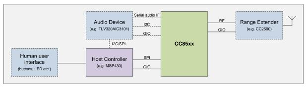
Figure 43 – Host-controller operated system
