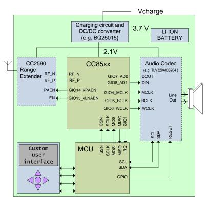
Figure 4 - Application block diagram for wireless headphone with host-controlled operation
