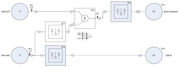
Figure 40 – USB HS 1 Headset Topology 1 Device Block Diagram
