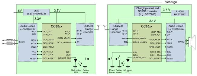
Figure 2 - Application block diagram for basic wireless headphone
