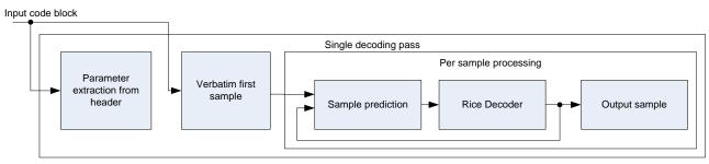
Figure 33 – SLAC decoding (16-bit)
