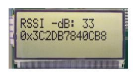
If the boards are moved farther apart from each other, the RSSI will drop (since the value is negative, a higher number means lower RSSI). If they are moved closer together, the RSSI should rise.
