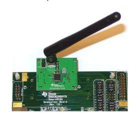
Next, mount the CC2541EMs firmly on to connectors P5 and P6 on the SmartRF05EB.
